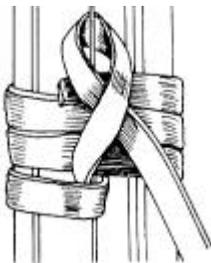
Again loop it round the tsuru, cross over and pass it under the last loop.
