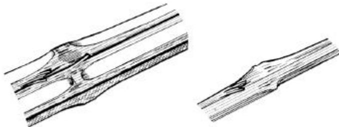
Scrape the splinters off with firm strokes from the hilt towards the tip, using a knife, file or a piece of glass. If you scrape from tip to hilt, the blade may dig into the bamboo.
