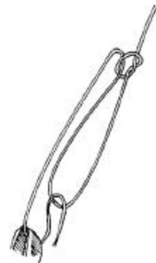
Pass the cord through the 'leather loop' on the hilt (kawa-himo); Thread it back through the komono. Pass it under the knot in the hilt's leather loop and pull it tight. Pull the cord taught with your right hand while you hold the komono down with the left.
