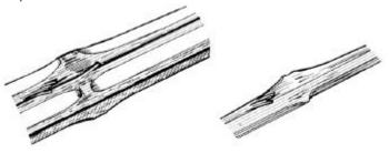
Scrape the splinters off with firm strokes from the hilt towards the tip, using a knife, file or a piece of glass. If you scrape from tip to hilt, the blade may dig into the bamboo.
